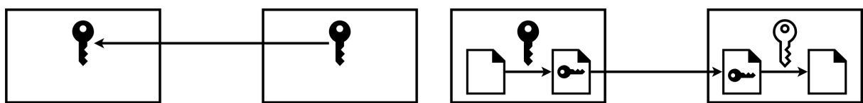
Figure 3.3: In asymmetric encryption the receiver sends its public key to the sender. Then the sender can encrypt information with the public key and send it to the receiver, who decrypts the ciphertext with another key – a private one.
