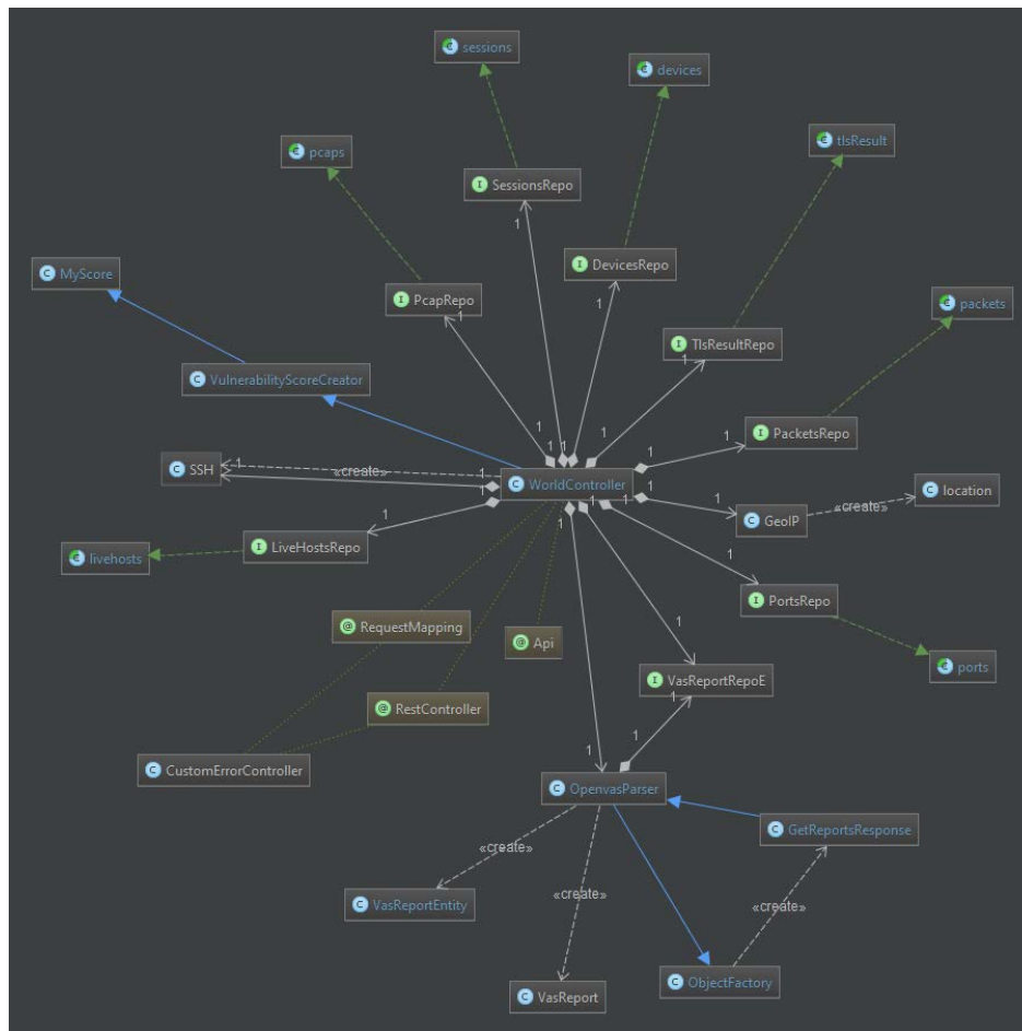
Figure 6. A class diagram with each module being a repository of entities mapped to the database.
